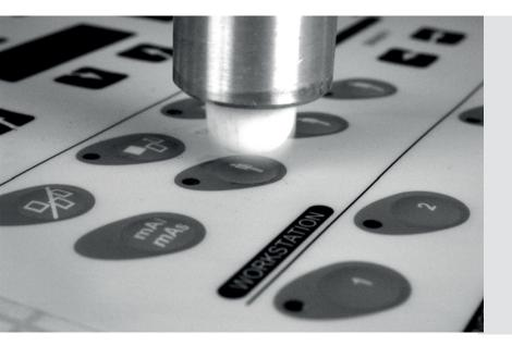
"CLICKTOUCH<sup>®</sup> retains essentially the same **ergonomic performance** as standard mechanical push buttons, but demonstrates the added benefits of being **dust and water tight**, as well as **chemically resistant**".
