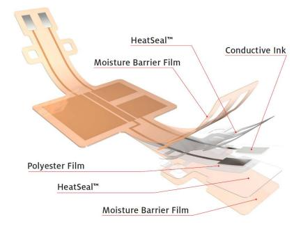
All basic polyester materials eventually allow moisture to pass through the material when continuously exposed to high humidity and temperature. With an exceptional MVTR tested at <.005g/ (m²\*day) this HeatSeal™ version can be designed into a membrane switch as an extreme moisture barrier bonding.
